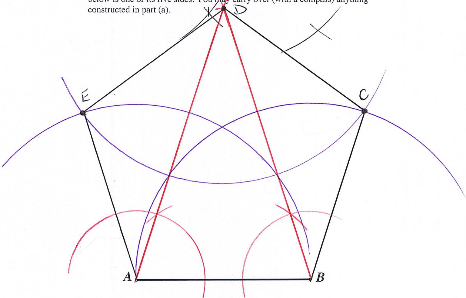
① Copy angle FCB ( $72^\circ$ ) to A and B to construct an acute golden triangle over AB. (in red)
